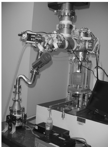
Fig. 6. High vacuum tribometer (photograph by Molina et al. [2, 25])
