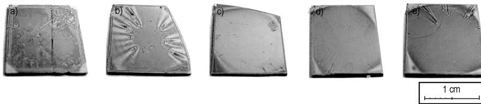
Fig. 1. Thin layers of spin-on dielectrics (HSQ polymer) coated at various rotational speeds: a) 1000 rpm, b) 2000 rpm, c) 3000 rpm, d) 4000 rpm, e) 5000 rpm
