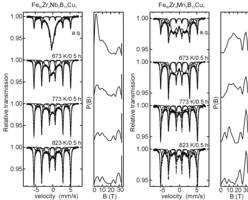
Fig. 1. Mössbauer spectra and hyperfine field distributions of the  $\text{Fe}_{82}(\text{Zr}_4\text{Nb}_3)\text{B}_{10}\text{Cu}_1$  and  $\text{Fe}_{80}(\text{Zr}_4\text{Mn}_3)\text{B}_{12}\text{Cu}_1$  alloys
