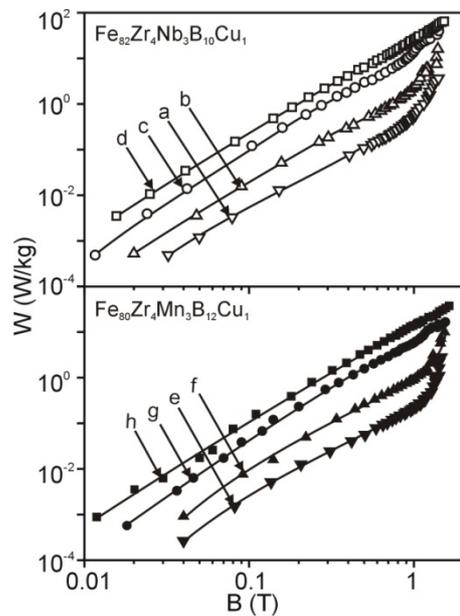
Fig. 3. Dependences of core losses ( $W$ ) on induction ( $B$ ) for the  $\text{Fe}_{82}(\text{Zr}_4\text{Nb}_3)\text{B}_{10}\text{Cu}_1$  alloy (a, b, c, d) and  $\text{Fe}_{80}(\text{Zr}_4\text{Mn}_3)\text{B}_{12}\text{Cu}_1$  alloy (e, f, g, h) after 0.5 h annealing at 823 K and 773 K, respectively, measured at the frequency of 50 Hz (a, e), 200 Hz (b, f), 1 kHz (c, g), and 2 kHz (d, h)
