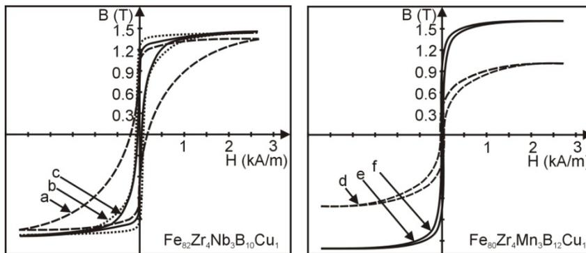
Fig. 2. DC hysteresis loops for the  $\text{Fe}_{82}(\text{Zr}_4\text{Nb}_3)\text{B}_{10}\text{Cu}_1$  (a, b, c) and  $\text{Fe}_{80}(\text{Zr}_4\text{Mn}_3)\text{B}_{12}\text{Cu}_1$  (d, e, f) alloys in the as-quenched state (a, d) and after 0.5 h annealing at 773 K (b, e) and 823 K (c, f)
