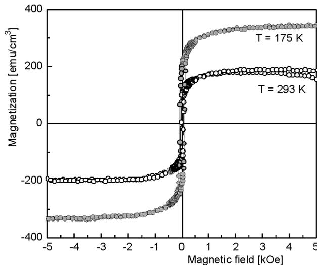
Fig. 2. Magnetization measured at 175 K and 293 K as a function of magnetic field for  $B2/L2_1$  ordered  $\text{Co}_2\text{CrAl}$  film annealed at 760 K (state 4)
