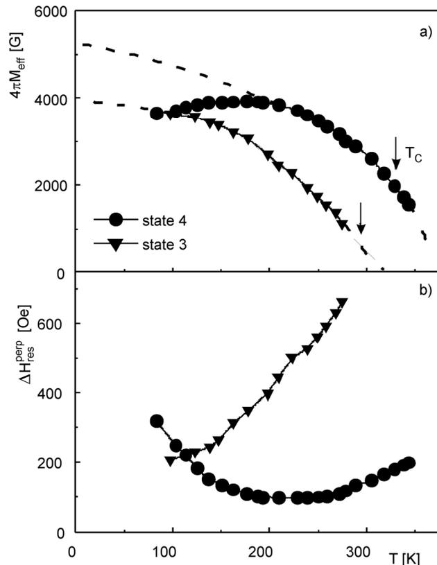
Fig. 4. Temperature dependences of the effective magnetization  $4\pi M_{\text{eff}}$  of the  $\text{Co}_2\text{CrAl}$  films annealed at 608 K (state 3) and 760 K (state 4) (a); FMR resonance linewidth  $\Delta H$  for the same films (b)
