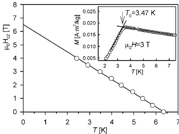
Fig. 4. Upper critical field  $H_{c2}(T)$  for  $\text{Mo}_2\text{Re}_3\text{B}_x\text{-Mo}_3\text{Re}_2\text{B}_x$  eutectic. The inset presents the way of determination of the critical temperature  $T_c(H)$  for a selected magnetic field (3 T in this case)
