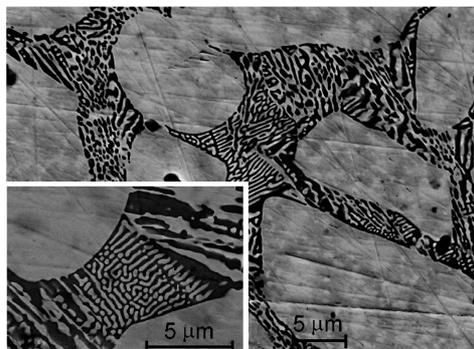
Fig. 1. The SEM micrography of  $\text{Mo}_2\text{Re}_3\text{B}_x\text{-Mo}_3\text{Re}_2\text{B}_x$  sample. Inset: the example of regular lamellar structure between globules of  $\text{Mo}_3\text{Re}_2\text{B}_x$  phase
