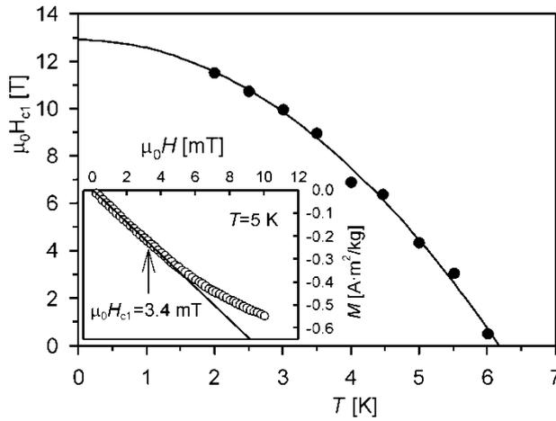
Fig. 5. The lower critical field  $H_{c1}(T)$  corrected for the demagnetising effect. The inset shows the magnetisation versus applied magnetic field  $M(H)$  for 5 K and the criterion for determination of  $H_{c1}(T)$ . The data in the inset are as measured (not corrected)
