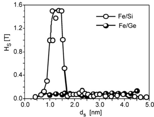
Fig. 2. The saturation field ( $H_s$ ) of Fe(3 nm)/Si( $d_s$ ) and Fe(3 nm)/Ge( $d_s$ ) vs. the spacer thickness of Si and Ge, respectively, at room temperature
