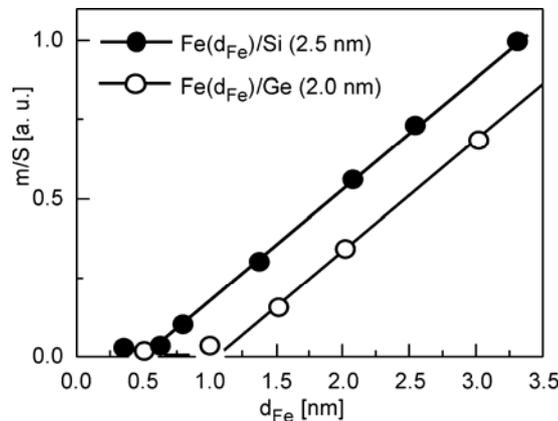
Fig. 3. Magnetic moment per surface area ( $m/S$ ) at room temperature for Fe( $d_{Fe}$ )/Ge (2 nm) and Fe( $d_{Fe}$ )/Si (2.5 nm) MIs as a function of Fe thickness
