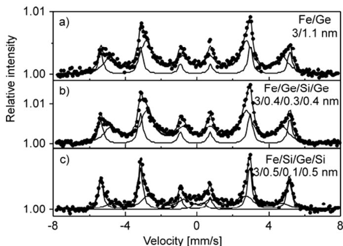
Fig. 5. Room temperature CEMS spectra for: a) Fe/Ge, b) Fe/(Si/Ge/Si) and c) Fe/(Ge/Si/Ge) MLs. Sublayer thicknesses are indicated
