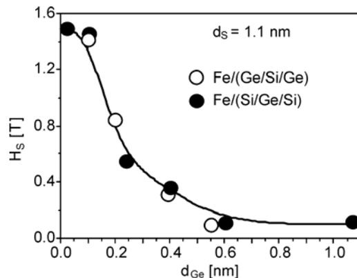
Fig. 4. The influence of Ge sublayer thickness on the value of  $H_S$  at room temperature
