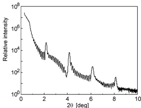
Fig. 1. An example of SAXRD spectrum recorded at room temperature for [Fe(3 nm)/Ge(2 nm)]<sub>15</sub> Mls
