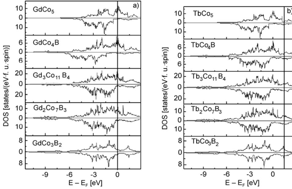
Fig. 1. The densities of states (DOS) of  $RCo_5$ ,  $RCo_4B$ ,  $R_3Co_{11}B_4$ ,  $R_2Co_7B_3$ , and  $RCo_3B_2$  compounds, where  $R = Gd$  (a) or  $Tb$  (b)
