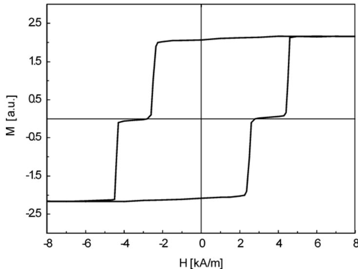
Fig. 1. A hysteresis loop of the 20 nm –Fe/2 nm – Zr/20 nm – Fe trilayer
