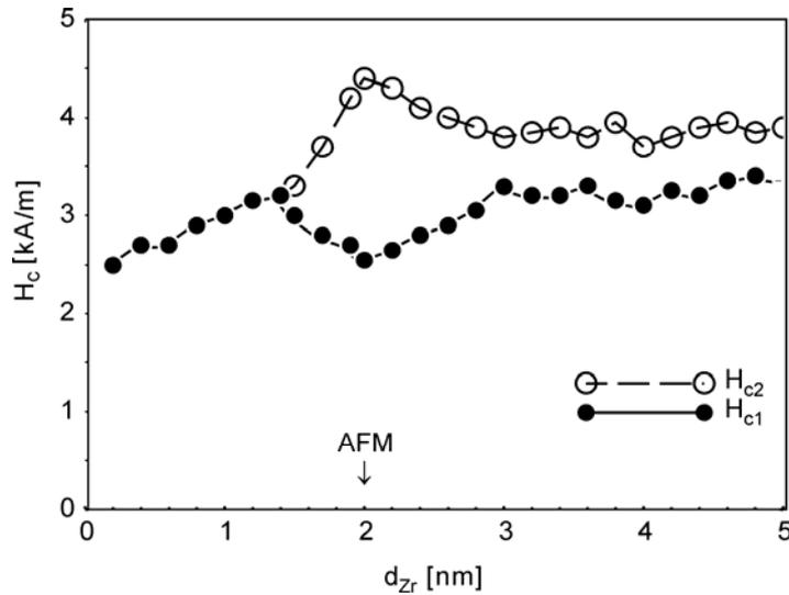
Fig. 2. Two different coercive fields  $H_{c1}$  and  $H_{c2}$  as functions of Zr interlayer thickness for a wedged 20 nm Fe/ $d_{Zr}$  Zr/20 nm Fe trilayer
