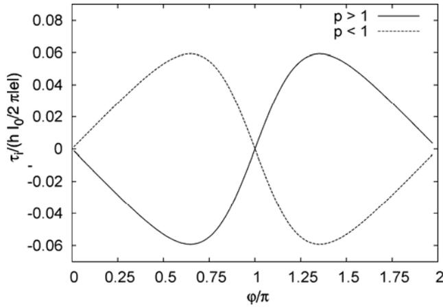
Fig. 2. Normalized torque acting on the island as a function of the angle  $\varphi$ , calculated for  $R_l^{p,+} = 25 \text{ M}\Omega$  ( $1 \text{ M}\Omega$ ),  $R_l^{p,-} = 1 \text{ M}\Omega$  ( $25 \text{ M}\Omega$ ),  $R_r^+ = 0.5 \text{ M}\Omega$  ( $0.1 \text{ M}\Omega$ ), and  $R_r^- = 0.1 \text{ M}\Omega$  ( $0.5 \text{ M}\Omega$ ), corresponding to
