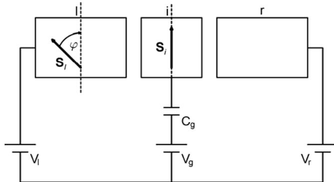
Fig. 1. A schematic diagram of the ferromagnetic single-electron transistor. The vectors  $\mathbf{S}_l$  and  $\mathbf{S}_i$  indicate the net spin moments of the left external electrode and the island, respectively
