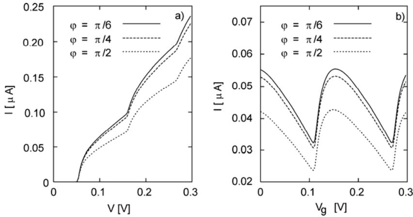
Fig. 3. Electric current as a function of the bias (a) and gate (b) voltages, calculated for  $p = 0.2$  and  $V_g = 0$  (a), and  $V_l = 0.043$  V,  $V_r = 0.043$  V (b). The other parameters the same as in Fig. 2
