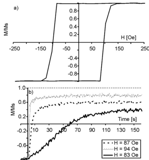
Fig. 1. Magnetic hysteresis loop for a cobalt film with a thickness of  $d = 1.5$  nm (a) and time dependences of film magnetization for different strengths of the applied magnetic field (b)
