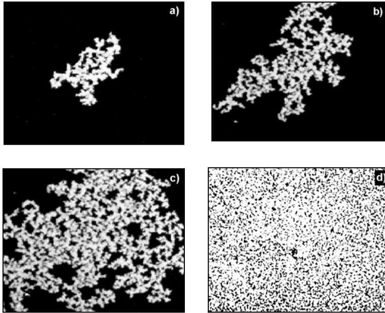
Fig. 2. Evolution of the dendritic domain structure in a cobalt film with a thickness of 1.5 nm. The sample was initially saturated by a field  $H < 0$  favouring “black” domains. Images after: a)  $H = 87$  Oe,  $\Delta t = 1$  s, b)  $H = 87$  Oe,  $\Delta t = 2$  s, c)  $H = 87$  Oe,  $\Delta t = 3$  s, d)  $H = 87$  Oe,  $\Delta t = 200$  s. The image sizes are  $0.11 \times 0.10$  mm<sup>2</sup>
