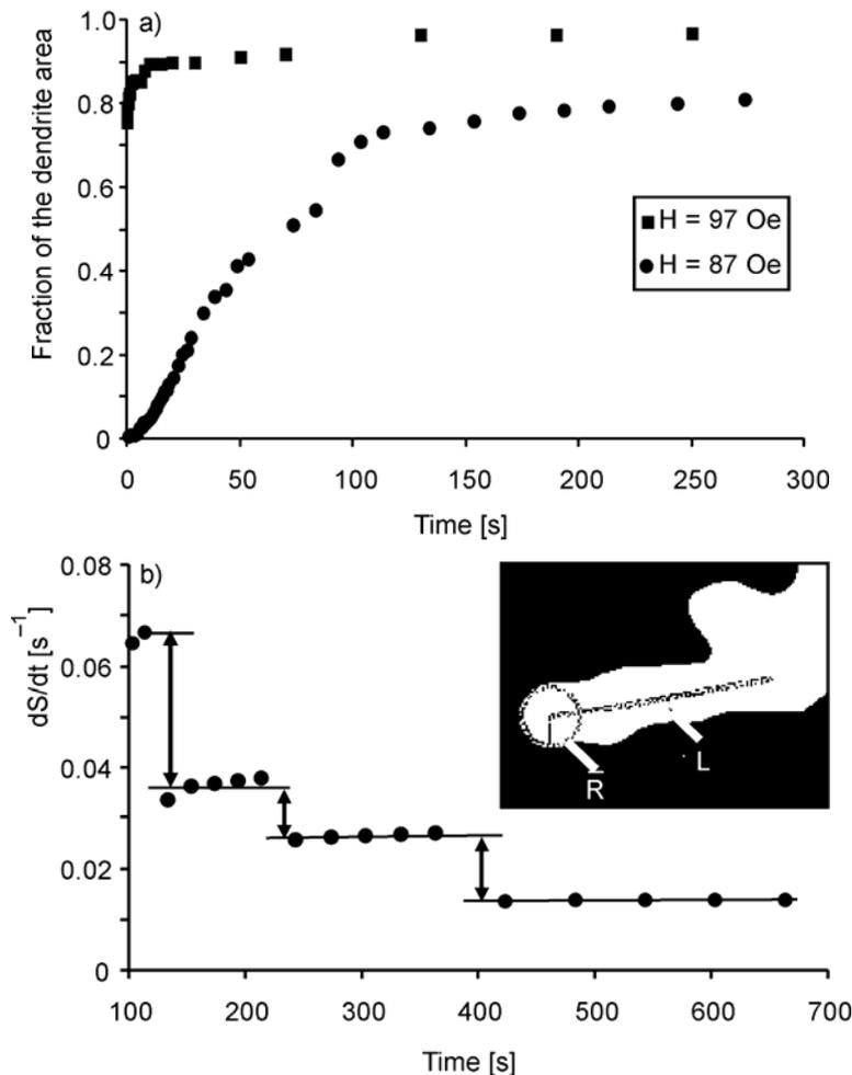
Fig. 3. Time dependence of the total reversed area fraction of domains for two amplitudes of the magnetic field (a) and time derivative of dendrite area (b),  $H = 87$  Oe.
